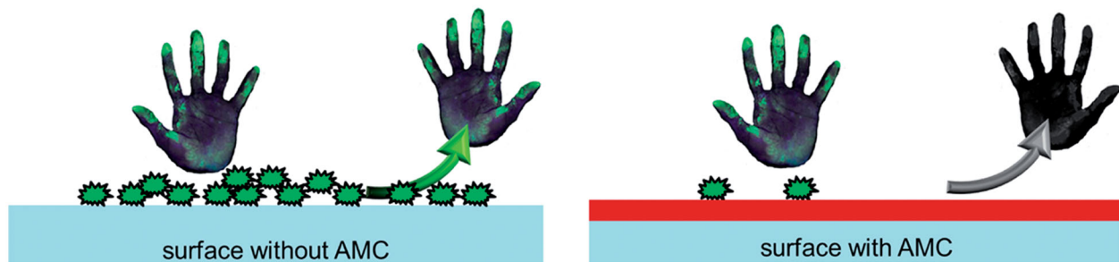
Figure 2. The number of MoV are reduced when frequently touched surfaces are equipped with an AMC. Consequently, the transmission of MoV should decrease.
