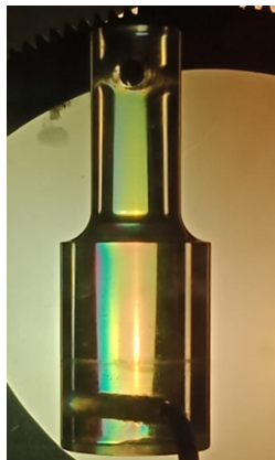
FIGURE 7. Image of the shouldered shaft under axial tension on photoelastic apparatus.
