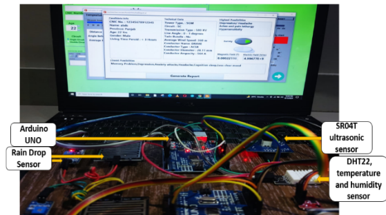
FIGURE 3. Sensors setup interfacing with software
