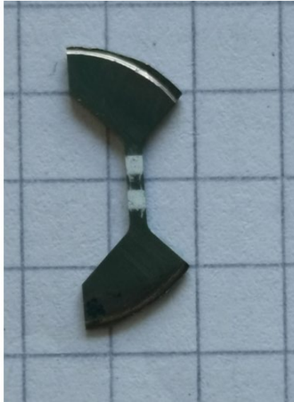
Figure 3.13 Schematic representation showing cutting position of tensile specimens in HPT-disks and specimens before test.
