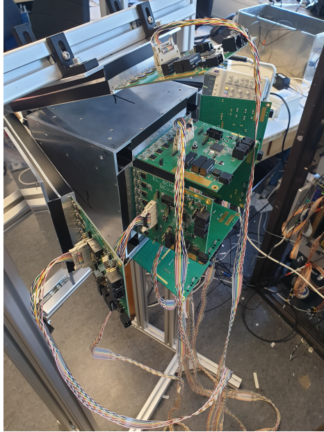
Figure E.3.: Photograph of the flat differential cables connected to the PCBs.
