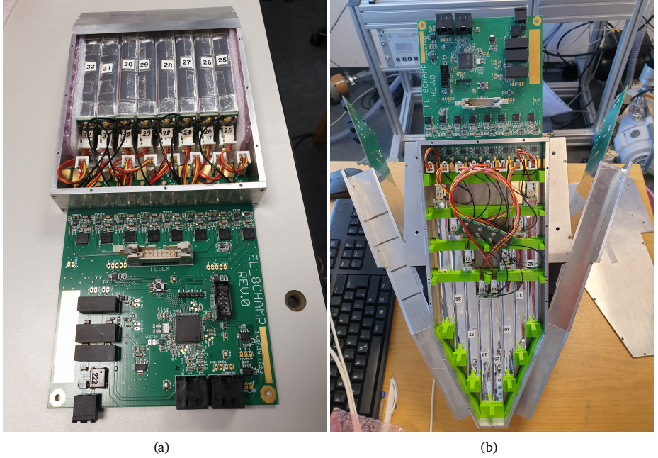
Figure 3.2.: Pictures of 8 BGO crystals in (a) a box from the back part and (b) a box from the front part of the pair spectrometer.
