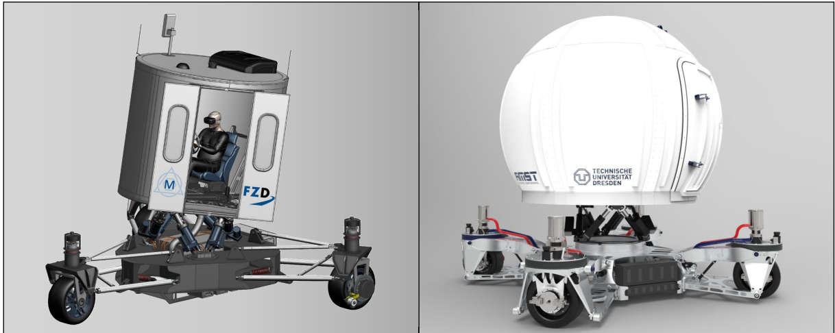
Figure 1-2.: Left: WMDS Design of TU Darmstadt with three wheel units. Right: Design of TU Dresden with four wheel units and turn table. 11
