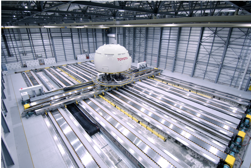
Figure 1-1.: Driving Simulator at Toyota's Higashifuji Technical Center in Susono City, Japan, built in 2007. The motion range is 35 m x 20 m. 5
