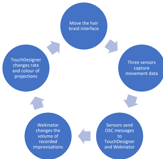
Figure 38: Diagram of Hél čhaŋkú kiŋ ħpáye (There lies the road) computer system.
