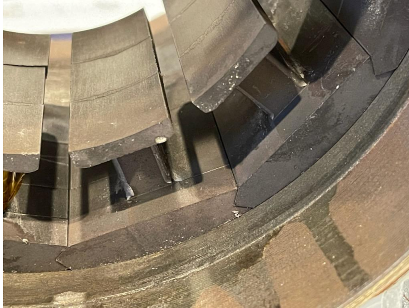
Fig. 4-22. Stator of the motor being prototyped
