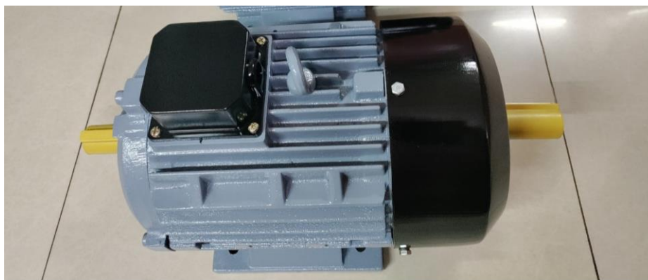
Fig. 4-20. Frame of the motor being prototyped.
