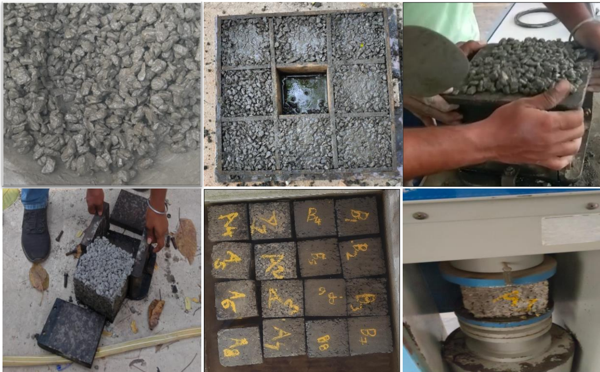
Fig. 5. Pervious concrete mix, sample preparation, curing and testing involved in the study
