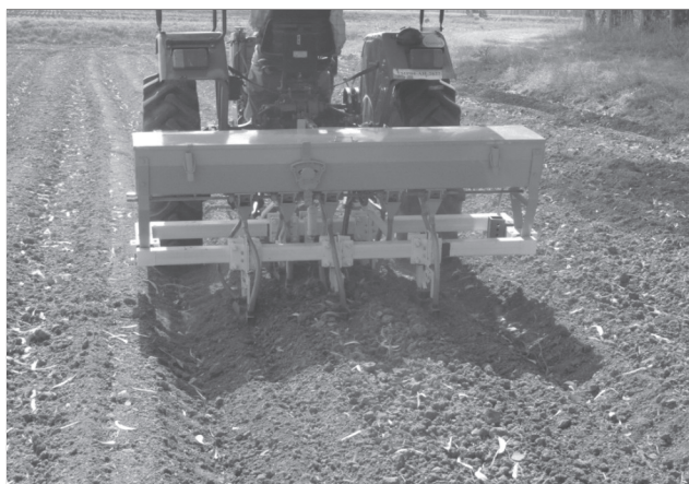
Fig 1 Wheat sowing with differential depth furrow opener on raised bed
