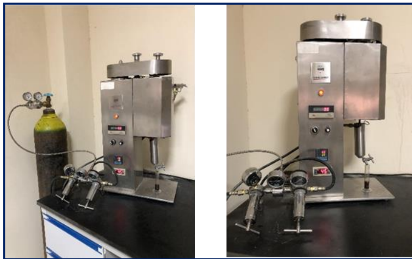
Figure 5: Dynamic HPHT filter press apparatus
