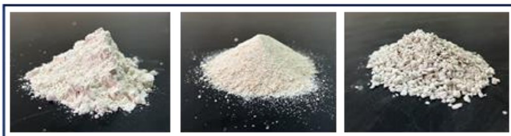
Figure 4: Fine, medium and coarse sized of CaCO 3 LCM
