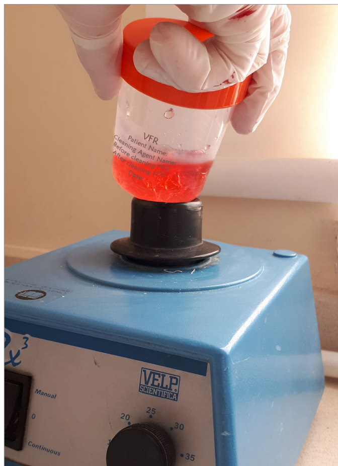
Figure 10. Homogenization of the VFR sample and Trypsin-EDTA in a vortex mixer and taking 1 ml of Trypsin-EDTA solution
