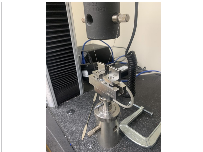
Figure 2. Tensile strength setup of the specimen
