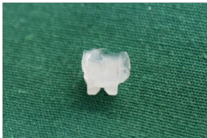
Figure 5. Peel off effect: entire composite is on the bracket surface after debonding of specimens immersed in glutathione (group III)
