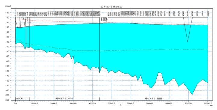
Fig. 5. Tool D1: Enhanced surge 'control', (high tide plus wind surge from C2), shown in cross-section up to the Thamesmead embankments (a realtime representation using MIKE11<sup>TM</sup>).
