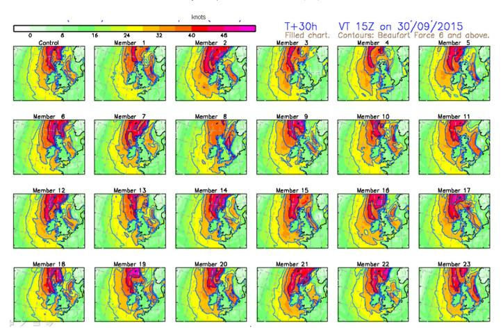
Fig. 4. Tool A5: weather predictions made72 h before predicted high tide: the 'control' wind map, alongside 23 ensemble members for the time interval covering the predicted high tide. (Original shaded in colour range from green to red). (c) Crown Copyright.
