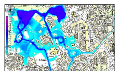
Fig. 6. Tool F3: Computer simulation of inundation of the Thamesmead embayment onto an OS map, using data available from tools E and D4, 24 h ahead of anticipated high tide. Real-time simulation using LiDAR DEM of the embayment, using a two-dimensional hydrodynamic model.
