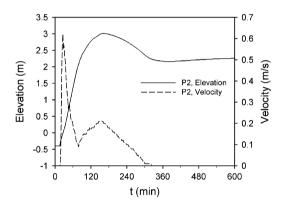
Fig. 7. Tool F4: Depth and velocity plots for any selected point within the Thamesmead embayment. These graphs can be shown alongside depth/velocity plan real-time simulations in plan.
