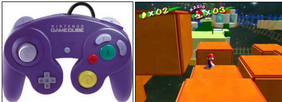
Fig. I.5. (a) Nintendo: GameCube controller, 2001 and (b) Super Mario Sunshine , 2002. The “A” button is used to jump and the yellow joystick to control the camera in Super Mario Sunshine . Both are controlled with the right thumb. It leads to odd situations when the game requires the player to jump from platform to platform while simultaneously controlling the camera in order to make sense of the surrounding.
