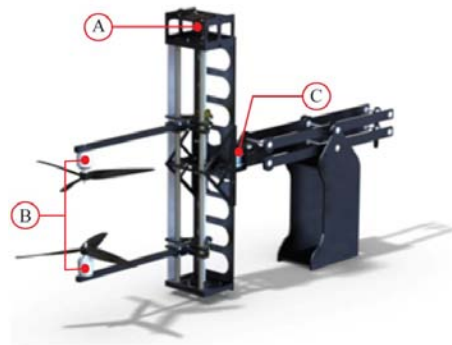
Figure 5 – Co-Axial Test-Rig in Situ: A) EMG30 motor, B) AXI-2217/20 motors, C) Yaw sensor.
