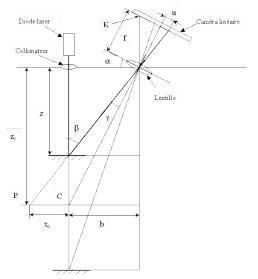
Figure 8. Triangulation methods for distance measurement [10]
