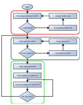
Figure 8. Arduino A flow chart
