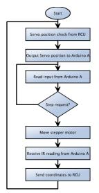
Figure 9. Arduino B flowchart
