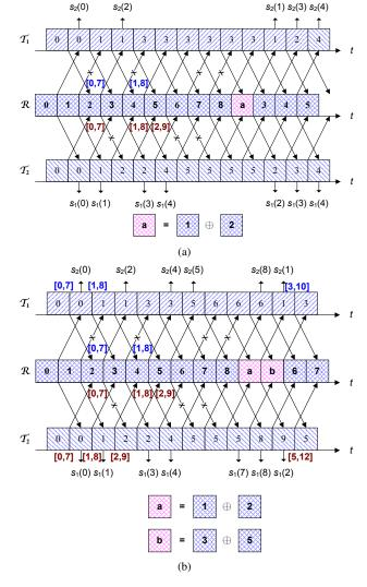
Fig. 4. BC phase with: (a) Improved NC-based GBN ARQ, (b) Improved NC-based SR ARQ,
