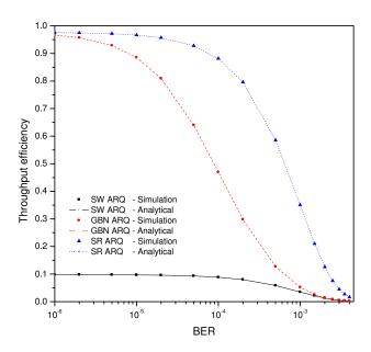
Fig. 5. Throughput efficiency of MA phase.
