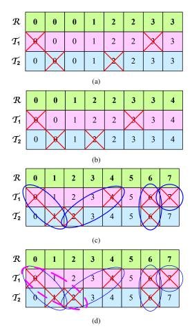
Fig. 3. BC phase with: (a) Memoryless ARQ, (b) Typical ARQ, (c) NC-based ARQ, and (d) Improved NC-based ARQ.
