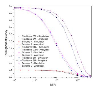
Fig. 7. Throughput efficiency of two-way relay network considering both MA and BC phase.
