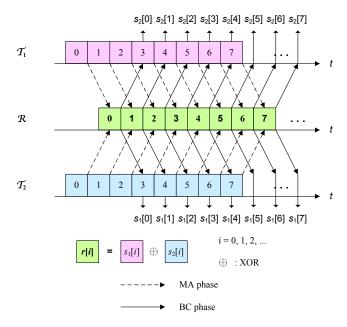
Fig. 2. Two-way relay channel with NC.
