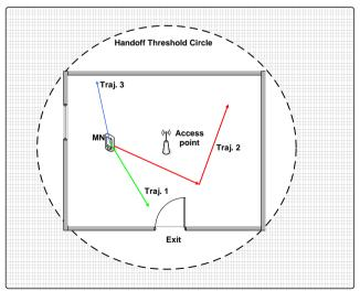
Figure 1. False handover triggers due to topological boundaries
