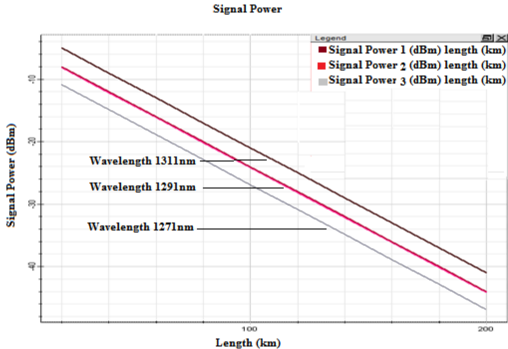
Figure 5-6: Signal power attenuation of 8 channels in SMF; dBm per km
