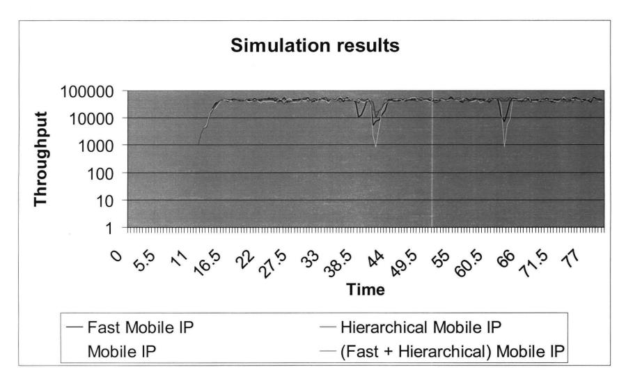
Figure 5-2 Simulation results Mobile IP
