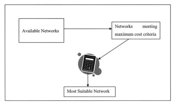
Figure 4-3 Network elimination based on cost
