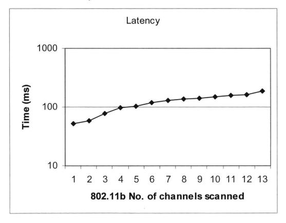
Figure 3-8 - Latency introduced by scanning for available channels
