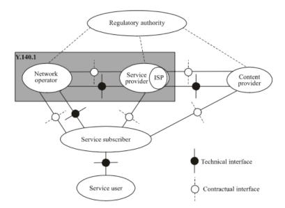
Figure 4.1: The ITU Recommended Network Parties
