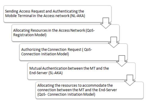
Figure 8.3: The Steps of Connection Security Model
