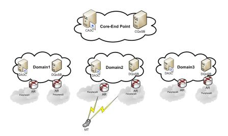
Figure 6.3: The Hierarchical Network Structure
