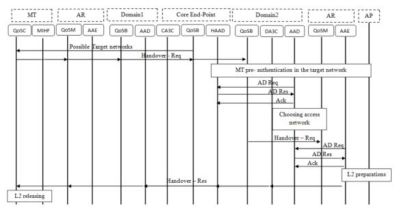
Figure 4.6: The Intra-Core End Point Handover Model
