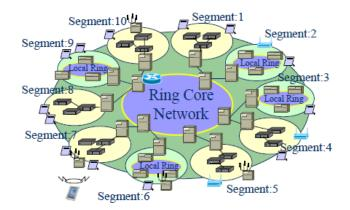
Figure 2.7: The Mobile Ethernet Network Structure (Kur05)
