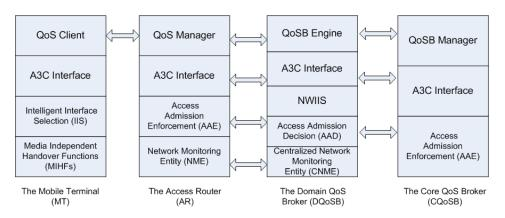
Figure 4.3: The Structure and Relationship Between the Network Entities
