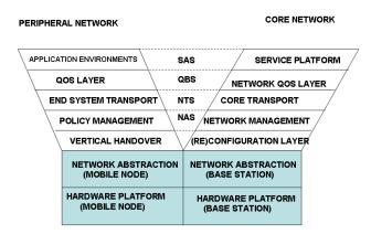
Figure 2.11: The Y-Comm Complete Structure
