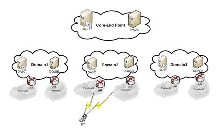
Figure 4.2: The Hierarchical Network Structure
