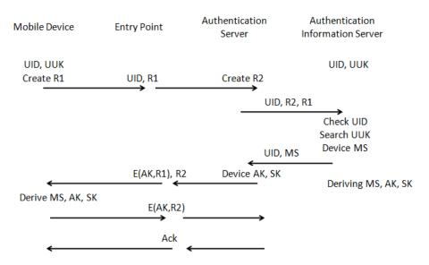
Figure 6.1: The Mobile Ethernet Protocol
