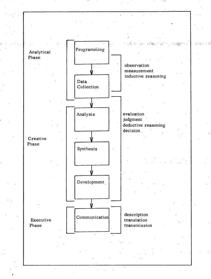
Fig. 9 Diagram of the main phases of design from Archer (Ref. 13).
