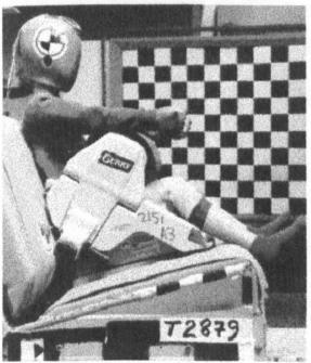
Figure 6.8 Shield type restraint
