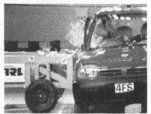
Figure 4.9 Exterior view of side impact occupant motion (adult shown)<sup>1</sup>
