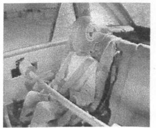
Figure 13.10 Struck side child occupant prior to impact, conventional CRS<sup>1</sup>
