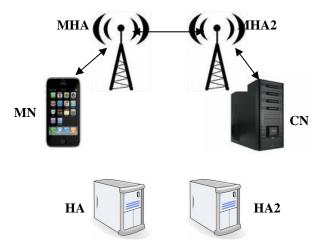
Fig. 6, Communication between mobile to mobile nodes via mobile home agents on points of attachment
