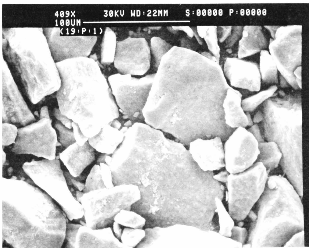
Figure 3-6 SEM photograph of 1-propanol most reduced IBA no.19, \text{MnOOH}_{1.0} .
