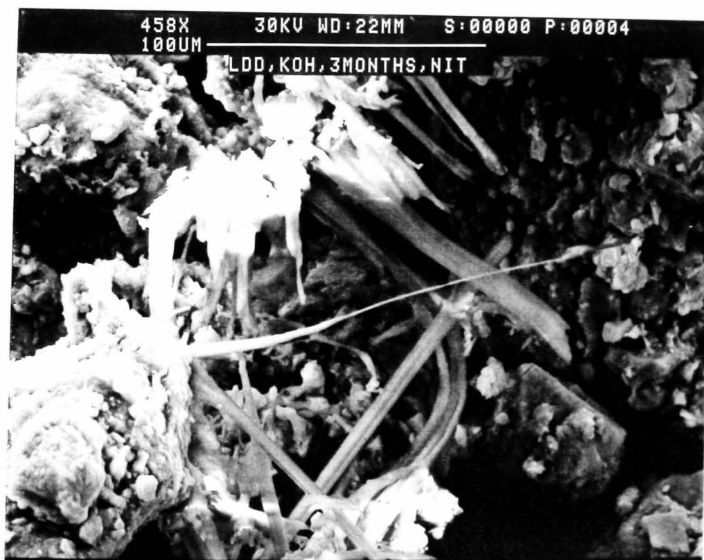
Figure 8-46 SEM photograph of H inserted IBA no.14 ( \text{MnO}_{1.505} ) after 3 months storage in 7M KOH, showing 'needle like' crystal growth.
