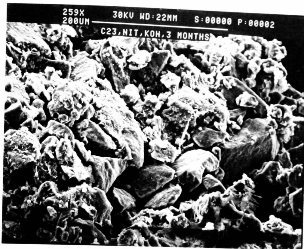
Figure 8-41 SEM photograph of H inserted IBA no.19 sample ( \text{MnO}_{1.544} ) after storage in 7M KOH for 3 months under \text{N}_2 .
