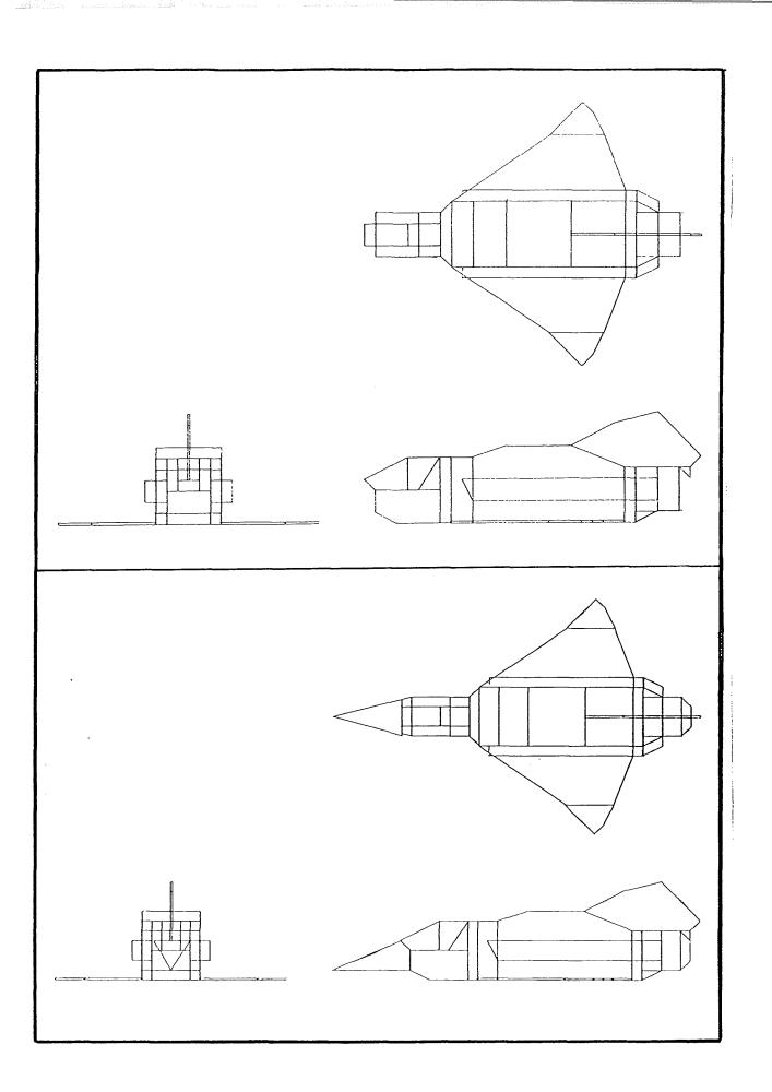
fig. 25. Two orthographic drawings of Howard Peters' spacecraft without the nose and complete with the nose.
