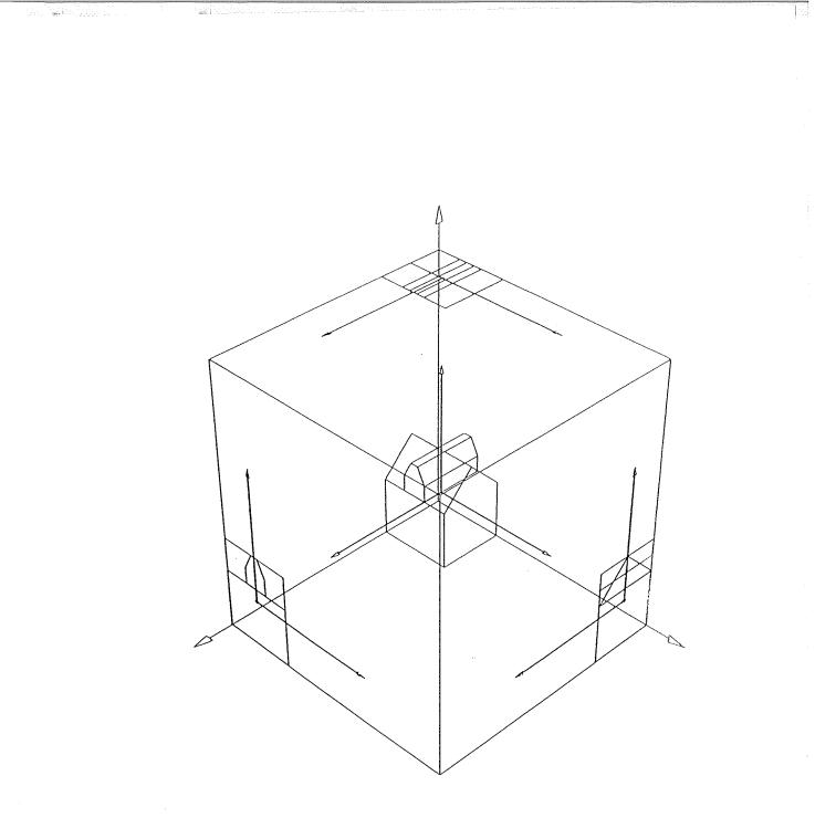
Fig. 14. A house in a glassbox. The house has 3D solid axes and in contrast to fig. 13. the axes are central to the house. It is intended to add 3D letters (X, Y, Z) to the program at a later date.
