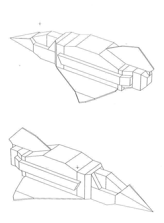
fig. 26. Two perspective views of Howard Peters' spacecraft rotated 180 degrees, these views reveal an error in the data for the nose that is not so easily noticed in the orthographic views.
