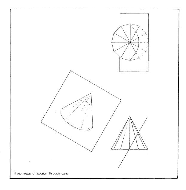
Fig. 22. Orthographic view and auxiliary view of a parabolic section through a right cone. Note the drawing is an orthographic view of three 12 sided models of cones and three planes as arranged in fig. 21.
