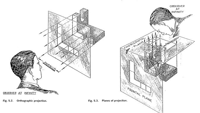
Fig. 24. Use of a man to help communicate the idea of orthographic projection. LUZADDER (1968, p. 82)
