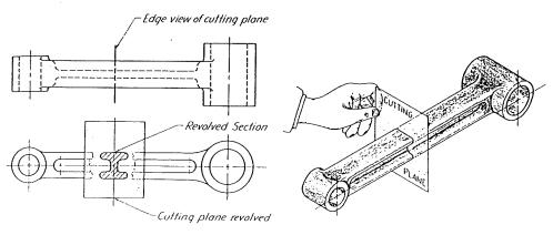
Fig. 9.9. A revolved section and cutting plane.
