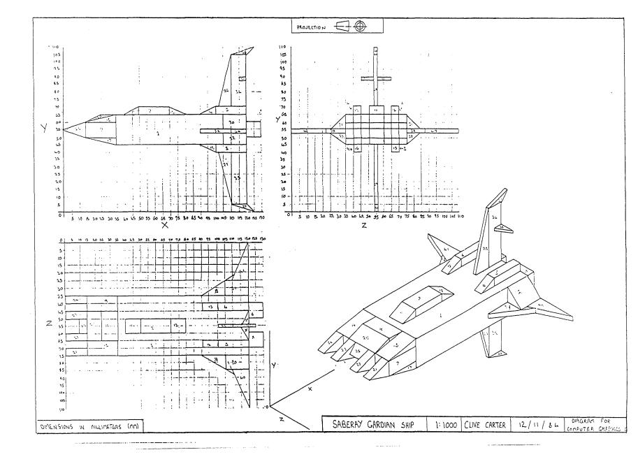
Fig. 57. isometric Saberay Gardian pictorial view. (sic) The of c) Ship by Clive Carter orthographic and original was drawn on A3 plain paper.
