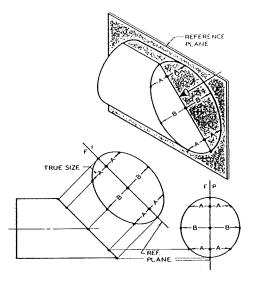
Fig. 5–86. Construction of an auxiliary view of an object requiring that a series of points be plotted. Since the object is symmetrical, the reference plane is positioned through its center.
