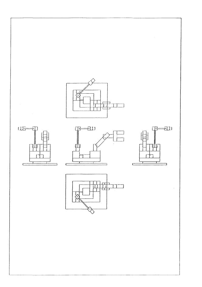
fig. 18. Five orthographic views of Howard Peter's robot showing rotation of the arms. Several drawings could be generated similar to this one with varying rotation to help pupils understand the foreshortening effect of rotation in the orthographic views.
