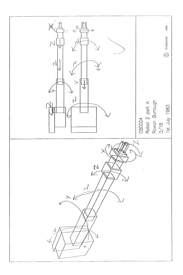
Fig. 47. Robot 2 part A. Plot used to label those component parts which are to be defined as sub-assemblies and for indicating rotational freedoms.
