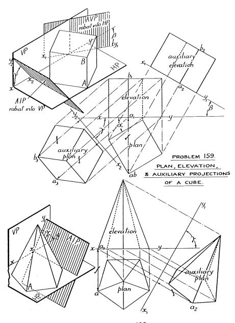
PROBLEM 160. PLAN, ELEVATION, & AUXILIARY PROJECTION OF A RICHT PENTAGONAL PYRAMID.
