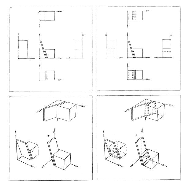
Fig. 25. Four frames showing five-view orthographics and the spatial arrangement from which the orthographic views have been derived.
