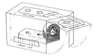
Fig. 5–81B. The projection planes are opened into a common plane to represent the plane of the drawing paper.
