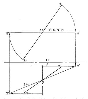
Fig. 10-10. The axis of revolution used to find the true-length view of a line can be placed anywhere on the line to be revolved. In this case a vertical axis was placed through point O of line *GH*.
