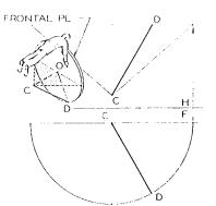
Step 1: The front view of line *CD* is used as a radius to draw the base of a cone with point *C* as the apex. The top view of the cone is drawn with the base shown as a frontal plane. The axis, *CO*, is perpendicular to the frontal base.
