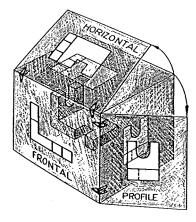
Fig. 5.5. The revolution of the planes of projection.
