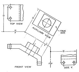
Fig. 5-848. Construction of an auxiliary view of the object shown in Fig. 5-84A as it would appear on your drawing paper.
