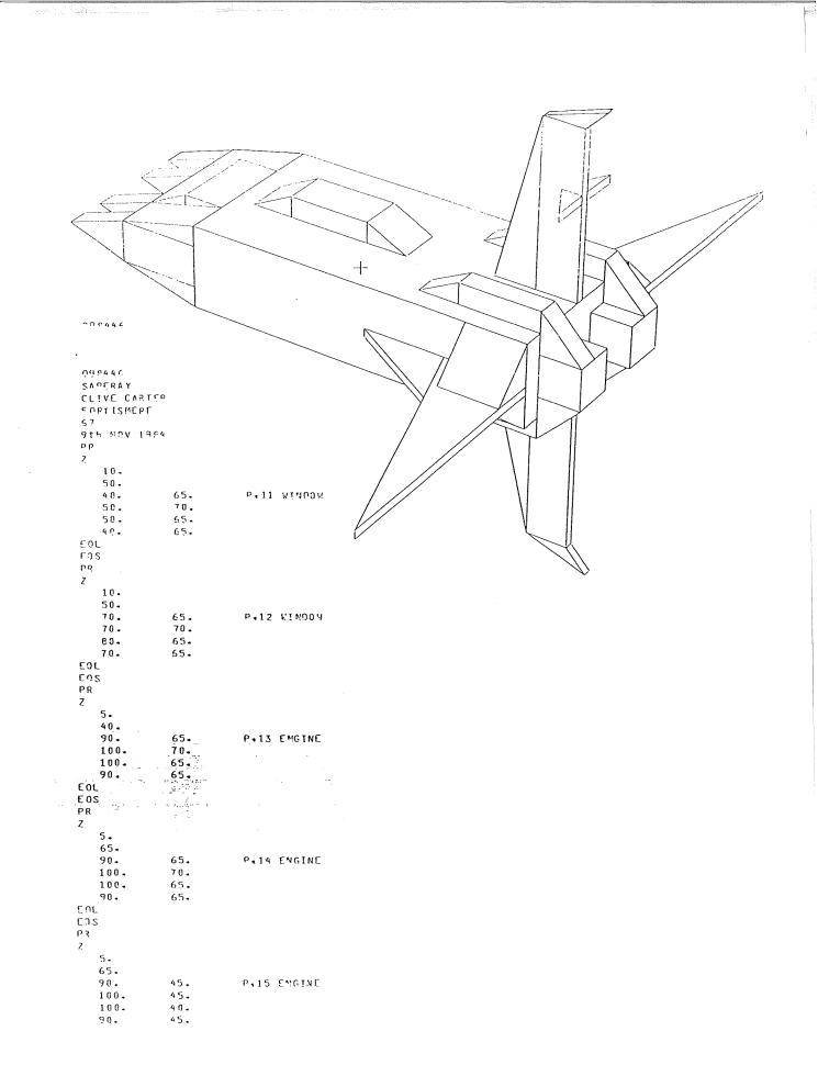
Fig. 59. perspective plot of Saberay and computer printout of part of the OBJECTSYN1 data file. Note the addition of identification for each part.
