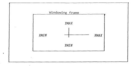
Any call upon *PLIT* will only generate drawings inside this boundary, clipping line segments against the four lines forming the rectangle.
