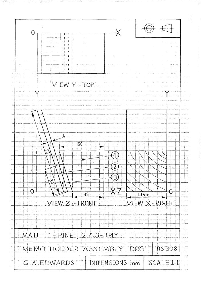
Fig. 23. Memo holder project. Orthographic views drawn to BS 308 except for the labelling of the axes.
