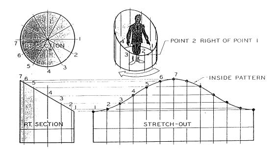
Fig. 12-10. Development of a cylinder.
