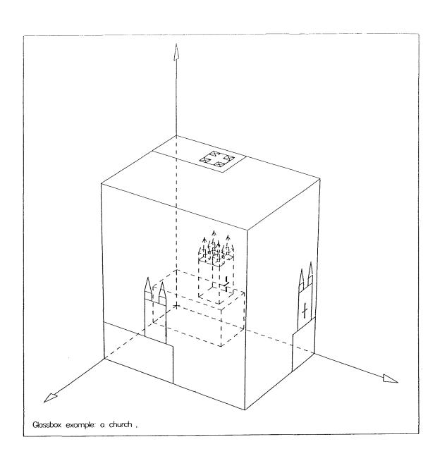
Fig. 15. A church in a glassbox. In this plot the glass is virtually opaque, resulting in the object being drawn in hidden detail mode. The views had to be projected slightly outside the sides of the box in order to be visible.
