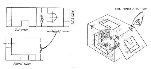
Fig. 6.7. The "second position" for the side view.
