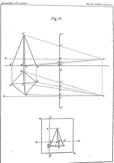
Fig. 45. Monge's application of descriptive geometry axioms to perspective projection, added to a late edition of *Géométrie descriptive* after his death. Compare with Fig. 18.
