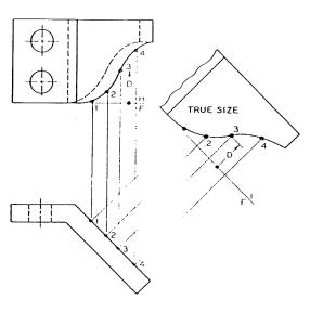
Fig. 5-83. Construction of partial auxiliary and principal views to depict an object.
