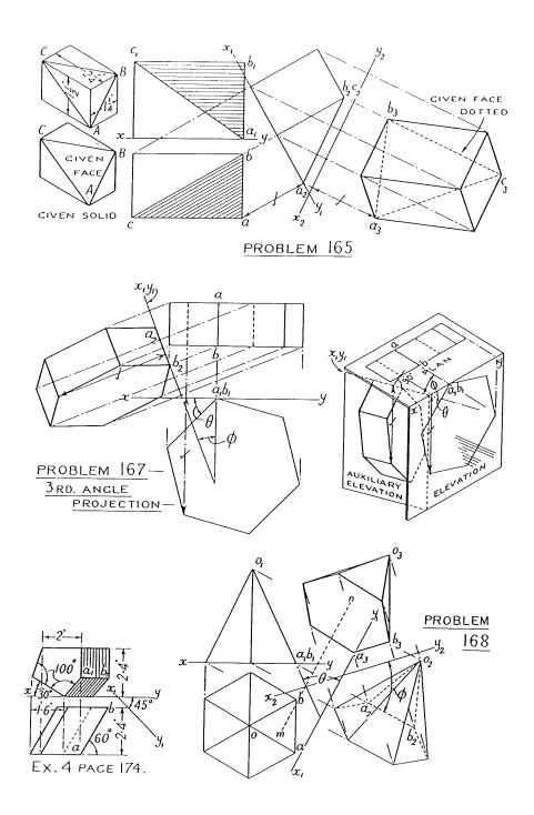
Fig. 2. Various problems which use the auxiliary view method. Problem 167 has a 3rd angle projection type isometric illustration to assist the learner. ABBOTT (1963, p.177)
