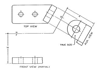
Fig. 5-81C. Construction of an auxiliary view of the object shown in Figs. 5-81A and 5-81B as it would appear on your drawing paper.
