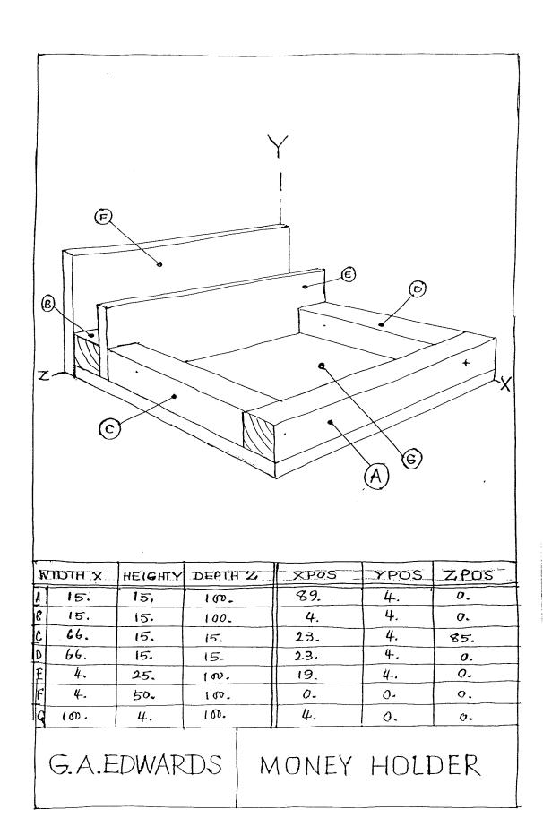
Fig. 26. Emergency Money holder project. Freehand pictorial view of the author's money holder example. The data for the computer was obtained solely by means of this pictorial view.
