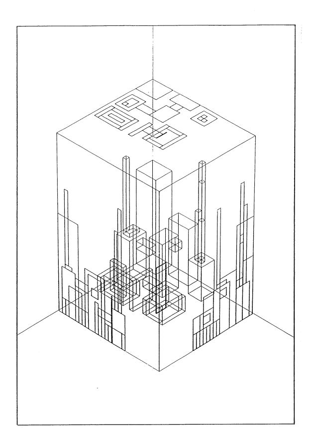
Fig. 17. A City Unit design in a glassbox. The GLASSBOX program has an option to plot the views in a different colour to the object in the box, this facility helps the pupil to distinguish the views.
