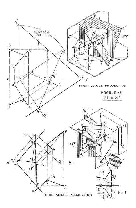
Fig. 1. Isometric scale illustrations in 1st and 3rd angle projection of related but not similar problems. The method depicted employs the trace of plane concept. ABBOTT (1963, P.215)
