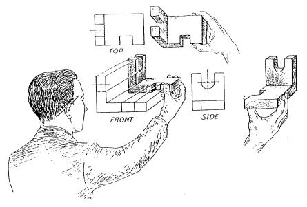
Fig. 6.2. Obtaining three views of an object.
