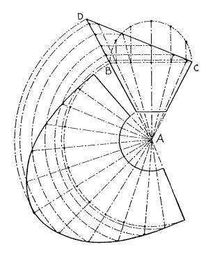
Fig. 10. Development of a watering can rose body in the shape of a frustrum of a right cone. This example shows how even a fairly simple component requires a lot of construction lines. DICKASON (1967, p. 38)
