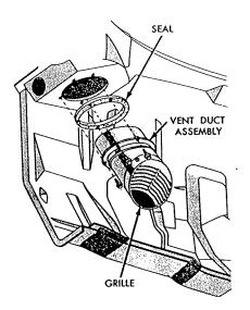
Fig. 12-11. This ventilator air duct was designed through the use of development principles. (Courtesy of Ford Motor Company.)
