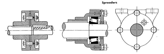
Fig. 5–96A. Parts not section-lined in an assembly—shafts, keys, bolts, and nuts. (Courtesy of ANSI; Y14.2–1957.)
