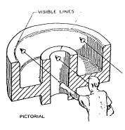
A. When a full section is taken through an object, you will see lines behind the sectioned area.
