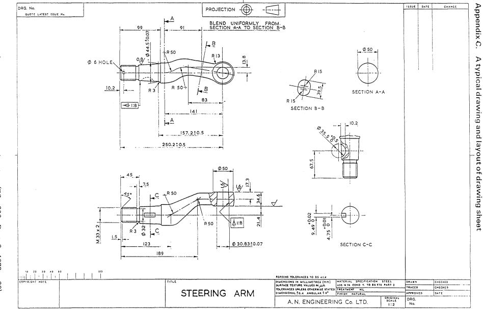
Fig.  $\overline{\mathfrak{A}}$  $\geq$ typical engineering drawing. (BS 308: Part 2: 1972, p39)
