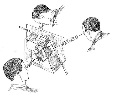
Fig. 8.1. Theory of projecting an auxiliary view.
