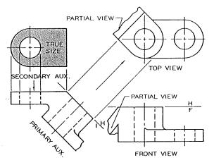
Fig. 5–87. An example of a secondary auxiliary view projected from a partial auxiliary view.
