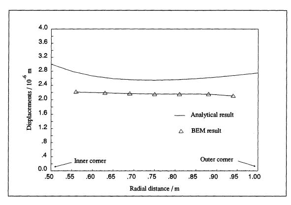
Figure 5.4: Comparison of horizontal displacements on surface S<sub>2</sub>.
