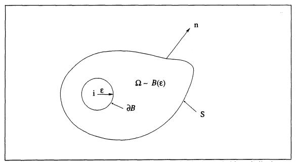
Figure 2.4: An elastic body with an interior point *i* surrounded by a ball of radius  $\varepsilon$ .
