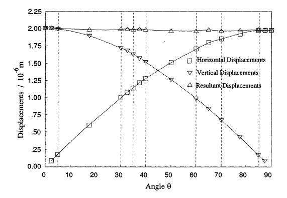
Figure 3.14: Surface displacements of unequally spaced quadratic elements with element subdivisioning. Fluctuations in the results are removed.
