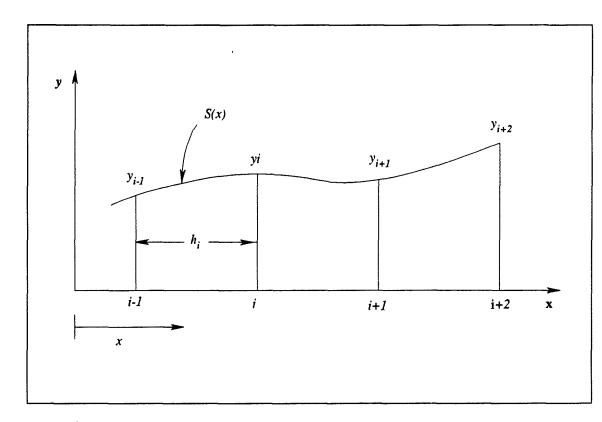
Figure 6.27: Parameters used for the spline fitting.
