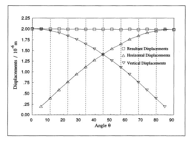
Figure 3.9: Surface displacements of equally spaced quadratic elements.
