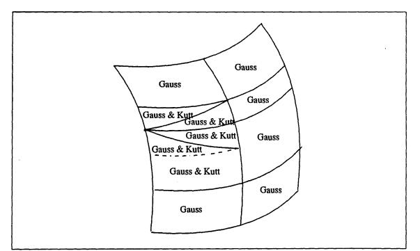
Figure 3.13: Unequally spaced elements. Distortion in the results are removed by the use of element subdivisioning.
