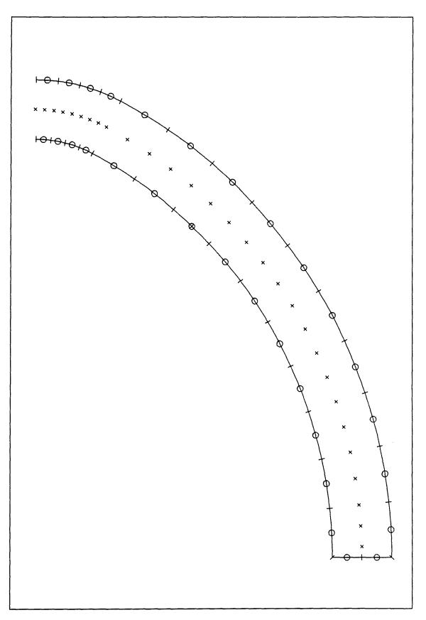
Figure 6.4: TheBEM mesh used for the cone with 10 mm wall thickness. Inner and outer surfaces were divided into 14 and the base surface was divided into 2 quadratic elements. Initially, the internal points were distributed along the mid-wall. Semi-continuous corner elements are not shown in this mesh.
