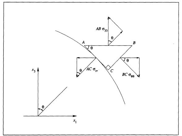
Figure D.2: Resolving forces to determine the stress  $\sigma_{33}$  in terms of the tangential stress  $\sigma_{\theta\theta}$ .
