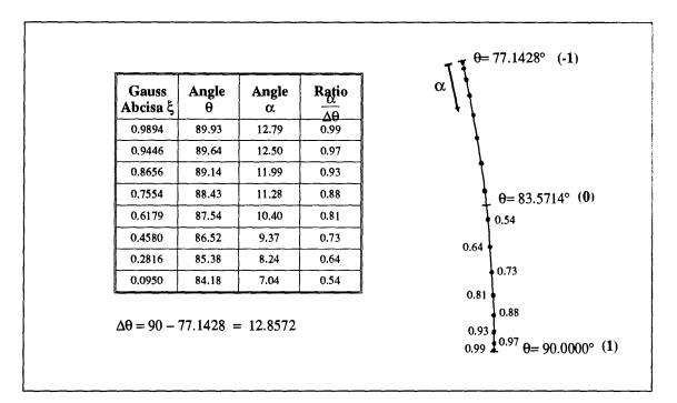
Figure 5.15: Mapping of Gauss points over the corner element on S<sub>1</sub>.
