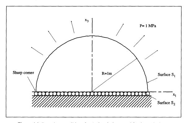
Figure 4.1: Boundary conditions for the hemisphere used for the analysis.
