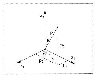
Figure 3.2: Components of the surface pressure p.
