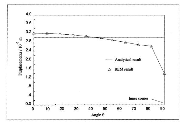
Figure 5.3: Comparison of resultant displacements on surface S<sub>3</sub>.
