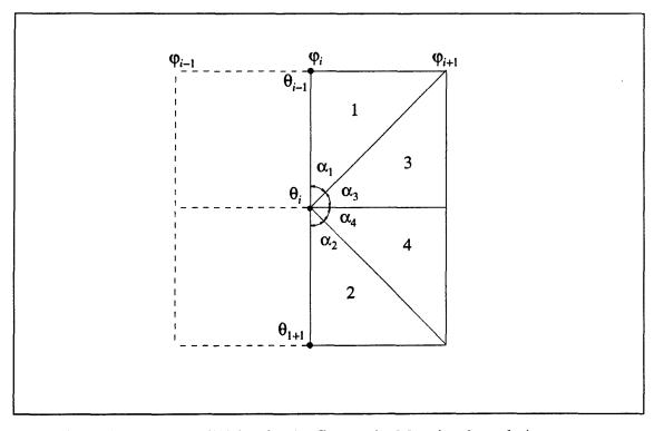
Figure 3.5: Element division for the Composite Mapping formulation.
