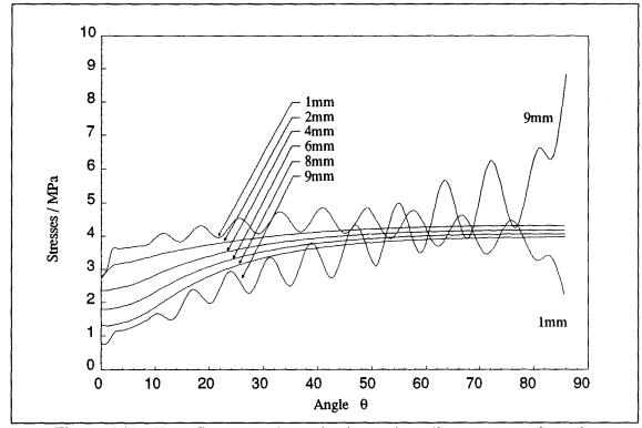
**Figure 6.18:** Hoop Stress  $\sigma_{\phi\phi}$  determined at various distances away from the inner wall surface. (Wall thickness=10mm)
