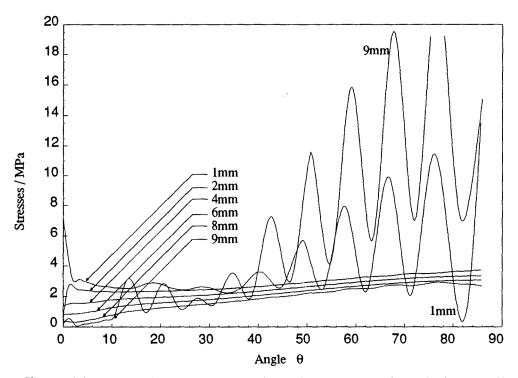
Figure 6.19: Von Mises stresses at various distances away from the inner wall. (Wall thickness=10mm)
