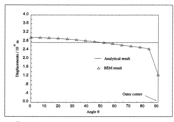
Figure 5.2: Comparison of resultant displacements on surface S<sub>1</sub>.
