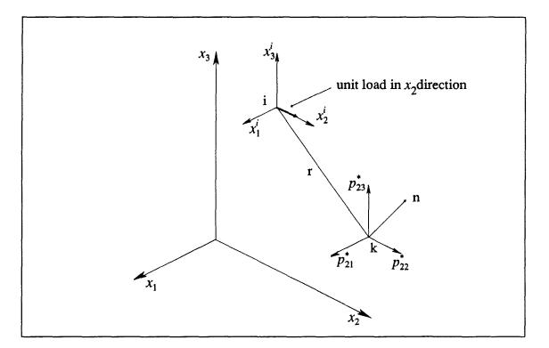
Figure 2.3: Coordinate system for the fundamental solutions.
