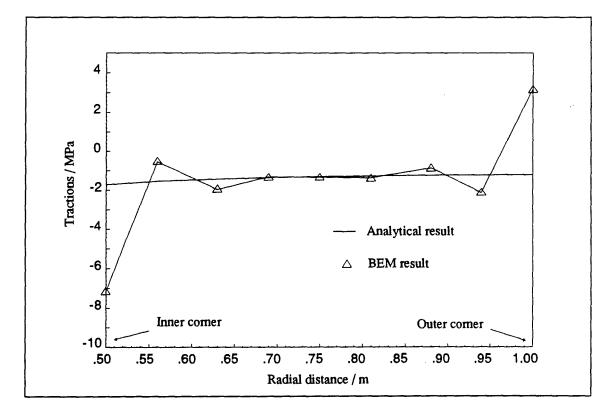
Figure 5.5: Comparison of tractions on surface S<sub>2</sub>.
