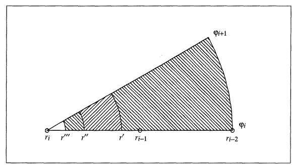
Figure 4.5: Integration scheme used for the central element of the S<sub>2</sub> surface (Drawing not to scale).
