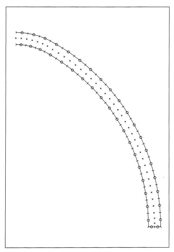
Figure 6.5: The BEM mesh used for the cone with 5 mm wall thickness. Inner and outer surfaces were divided into 19 and the base surface was divided into 2 quadratic elements. Initially, the internal points were distributed along the mid-wall. Semi-continuous corner elements are not shown in this mesh.
