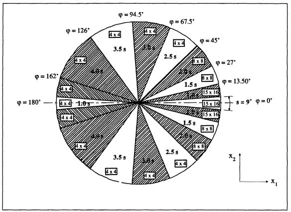
Figure 5.22: A typical allocation of segments in  $\varphi$  direction to reduce the CPU time by allowing incremental segment size based on the element length in  $\theta$  direction and also variable quadrature order for integration.
