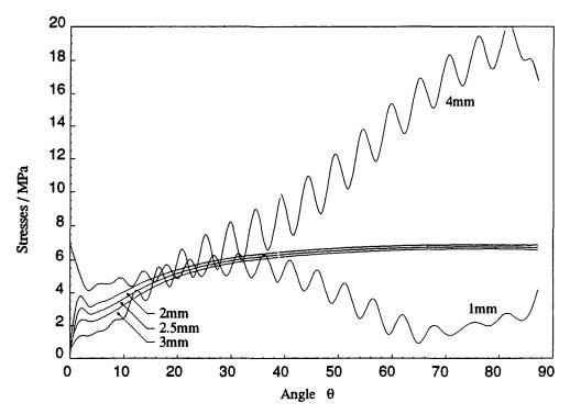
Figure 6.21: Von Mises stresses at various distances away from the inner wall. (Wall thickness=5mm)
