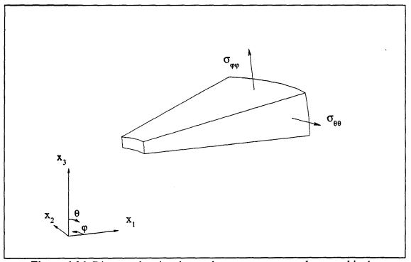
Figure 6.16: Diagram showing the two hoop stresses  $\sigma_{\theta\theta}$  and  $\sigma_{\phi\phi}$  used in the nodal stress comparison.
