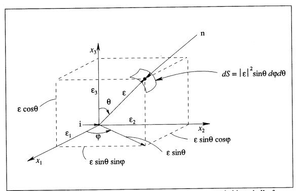
Figure 2.5: Geometry definition of an internal point surrounded by a ball of radius  $\varepsilon$ .
