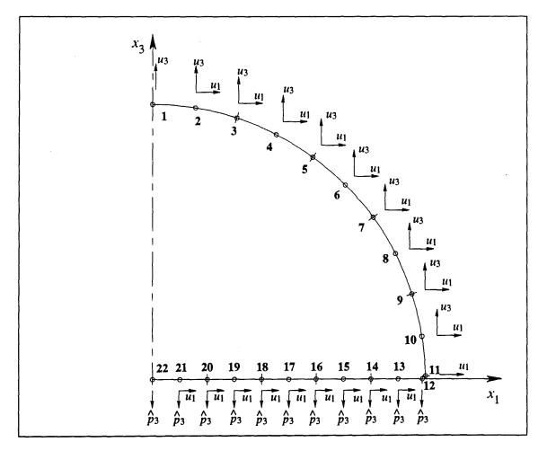
Figure 4.2: Descretization used for the hemisphere.
