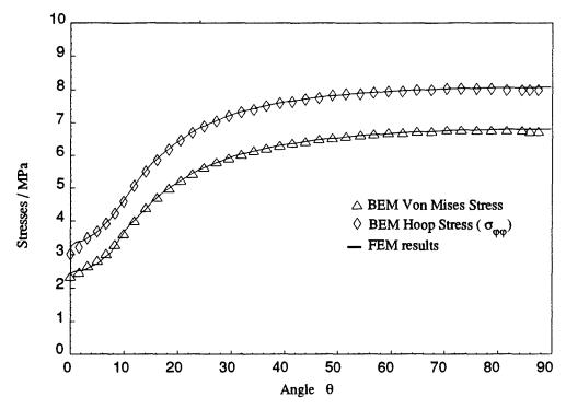
Figure 6.17: Comparison of BEM and FEM Von Mises and Hoop Stress  $(\sigma_{\phi\phi})$  at mid-wall of the cone. (Wall thickness=5mm)
