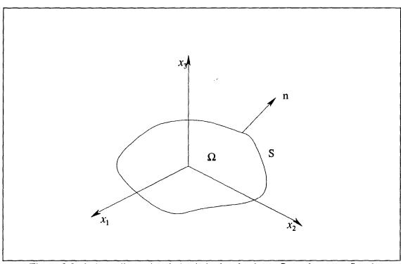
Figure 2.2: A three dimensional elastic body of volume  $\Omega$ , surface area S and a unit normal vector n.
