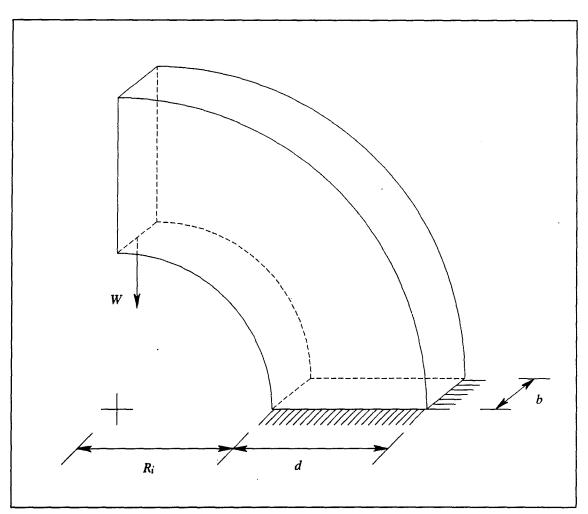
Figure C.1: A Curved beam used for the comparison of tangential stress  $\sigma_{tt}$  at angle  $\theta = 45^{\circ}$ .
