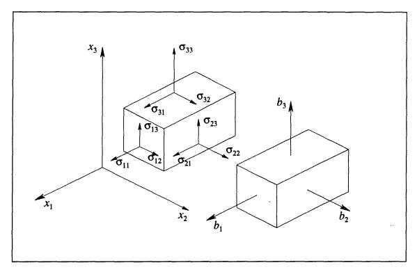
Figure 2.1: Stresses and body forces acting an a three-dimensional element.
