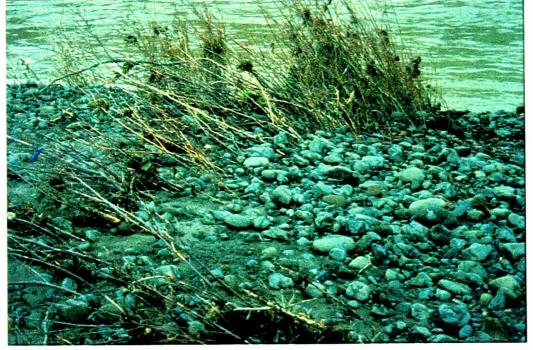
Photo 5.12. Sediment particles captured by baffles during 15 year flood, peak flow depth  $\sim 1$ m, photo taken 10 Jan 1995.
