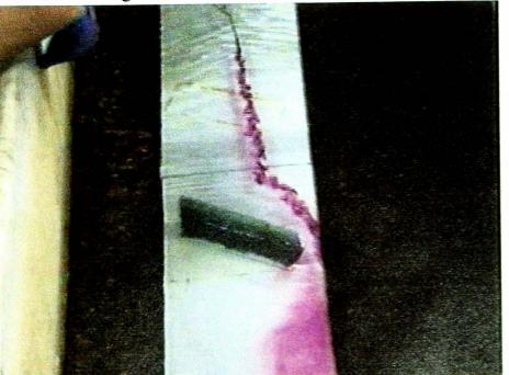
Photo. 7.1. Flume visualisation of the hydraulic separation point upstream of a single emergent, porous, vegetative filter.
