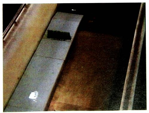
Photo 6.14. View of the final baffle design and simulated terrace in the flume.
