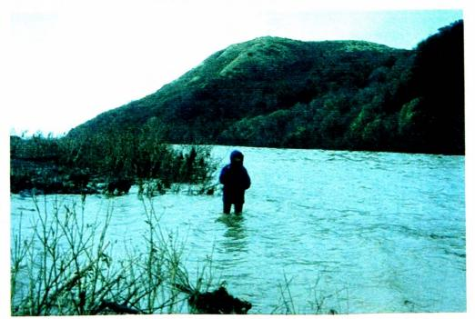
Photo 5.13. The author holding current meter, counting clicks for velocity measurements, velocity profile 4, 10 Jan 1995.
