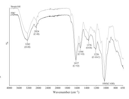
**Fig. 3.** FT-IR spectra of EPS from *Bacillus subtilis* 168 and FBC5 biofilms after 1 week of incubation at 37 °C. Upper spectrum, *B. subtilis* 168; lower spectrum, strain FBC5. FT-IR were conducted in replicas for each strain revealing identical peak patterns among preparations.
