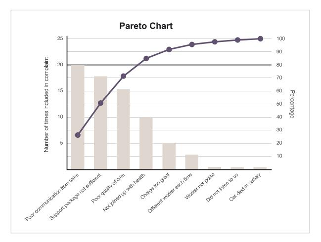
The purpose of the chart is to show the relative importance of each of a list of categories/ factors in relation to the specified unit of measure. In the context of improving quality, it is used to highlight the most common errors, the most frequent types of customer complaints, or the most complained about product or service etc. Effort is concentrated on solving the problems with the most frequent occurrence (towards the left hand of the distribution).
