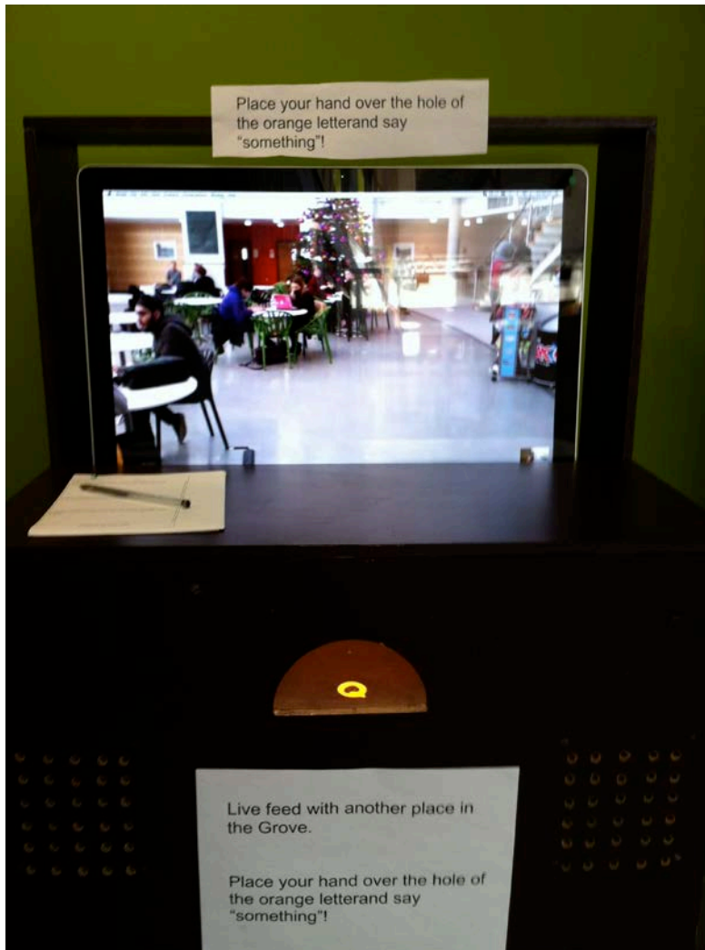
Figure 26: TT with holes for speakers, instructions and an orange sticker to mark the hole
