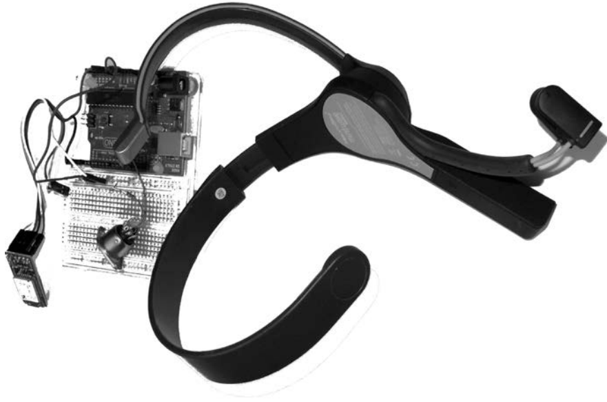
Fig. 2. The equipment used, Arduino, Bluesmirf and Mindwave.
