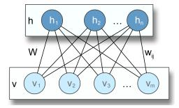
Figure 1: The RBM architecture.
