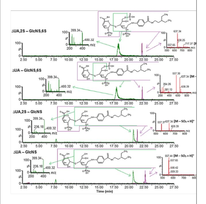
In contrast, the intact non-sulphated and *N*-acetylated disaccharide ions  $[M + H]^+$  were still detected at 65 °C. However, in-source fragmentation resulted in the loss of one or two sulphonic groups (Fig. 4). Thus, it appears that the sulphated disaccharides with sulphonic groups attached to N-position of glucosamine are relatively heat-labile compared to disaccharides sulphated at other positions. Also, at 65 °C derivatisation temperature, a peak
