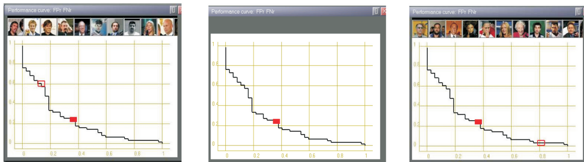
(a) Performance curve of the classification model with horizontal axis showing the false positive rate and vertical axis showing the false negative rate.
