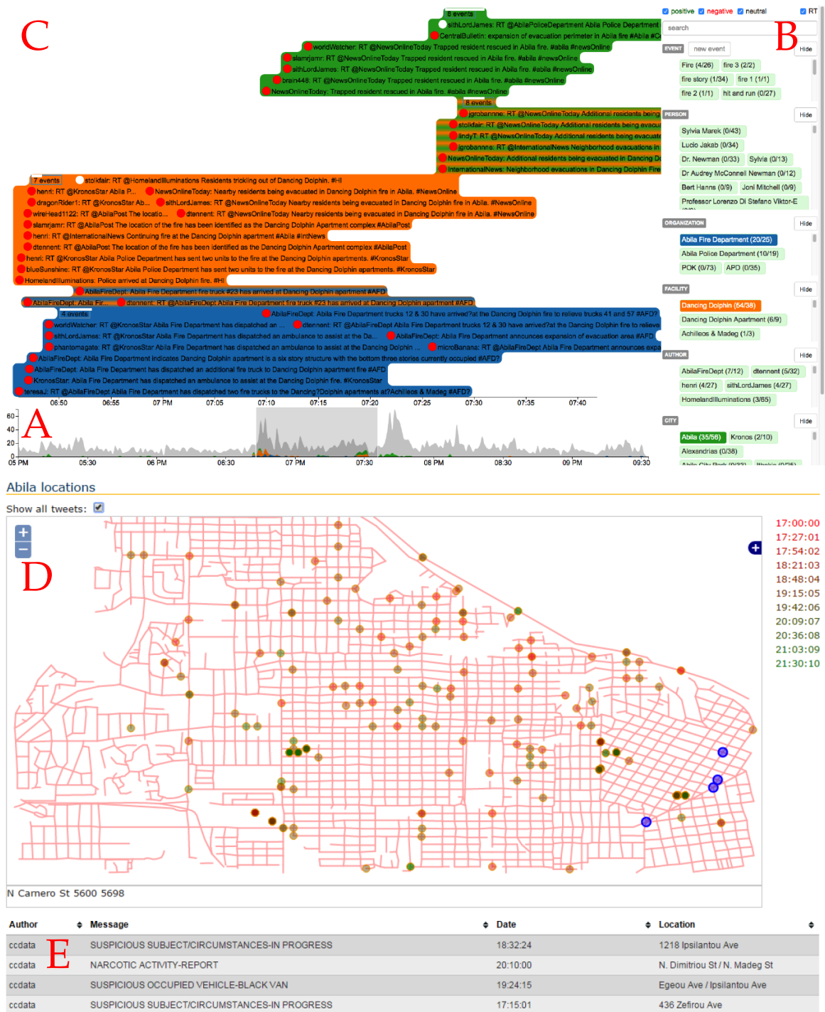
Figure 4.13: SAVI interface. A: Histogram showing the distribution of tweets. B: Extracted named entities organized by type. C: TimeSets displaying selected tweets. D: Map showing tweets with available geolocation. E: Details of tweets selected in the map.
