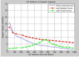
Figure 11. The Ergodic Capacity when the VPL = 40dB
