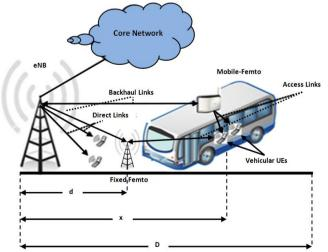
Figure3. eNB, Fixed & Mobile Femtos system model architecture
