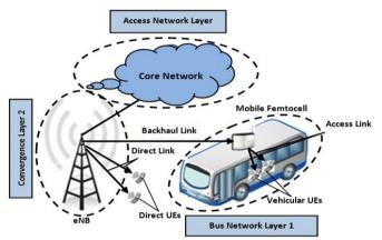
Figure2. Mobile Femtocell architecture with its layering system
