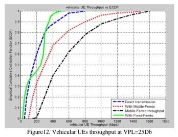
Furthermore, the black curve shows that the Mobile-Femtos themselves have a higher throughput around 500Kbps due to the additional gain in the received SINR on the backhaul link.
