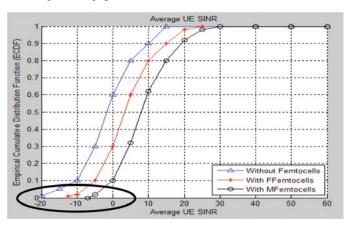
Figure 16. SINR of mobile UEs without & with FFemtocells/MFemtocell
