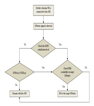
Figure 13. New connected UEs case 2
