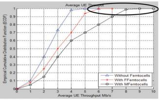
Figure 15. Average throughput of mobile UEs without & with FFemtos/MFemtos
