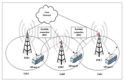
Figure 10. MFemto HO between two cells
