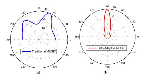
**Figure 2.** Different methods of measuring the angle of arrival. (a) Traditional MUSIC Algorithm; (b) self-Adaptive MUSIC Algorithm.
