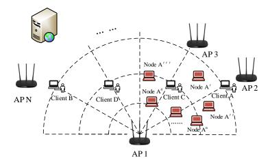
Figure 4. Sybil attack detection system of multiple detection APs.
