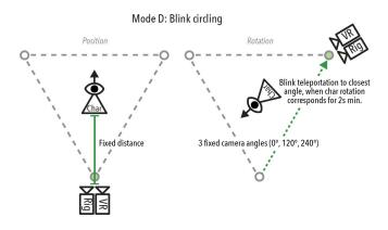
Figure 7: Mode D: Blink circling Visualization
