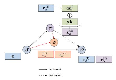
Fig. 1: System model of a CWRN in the presence of an eavesdropper.
