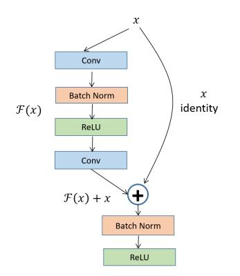
Figure 2. A typical residual block in a residual learning network Resnet [20] and its optimised version.
