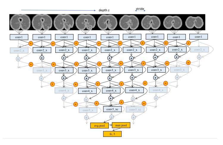
**Figure 4.** A block in the depth-Resnet that is applied in the paper. The outputs of conv5\_X are max-pooled in time and fed to the fully connected (fc) layer of the proposed depth-Resnet as shown in Figure 3(b) to classify 5 categories.
