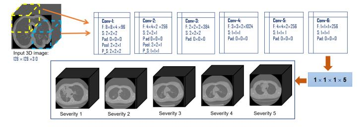
Figure 9. The architecture of the applied conventional 3D CNN network.
