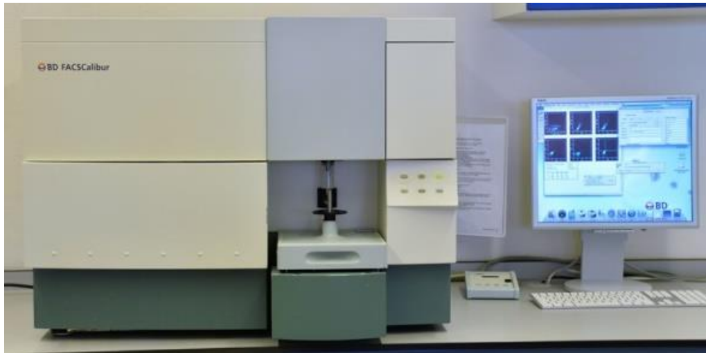
Fig 2.2.7: Representation of a BD FACSCalibur flow cytometer
