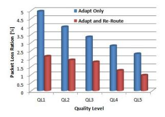
Fig. 6. Scenario 3 Packet Loss Ratio for Adapt Only vs. Adapt and Re-Route
