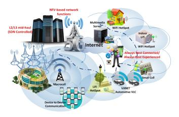
Fig. 1. SDN-based Heterogeneous 5G Environment
