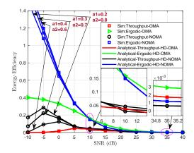
**Fig. 11**: Energy efficiency of two users for the PSR protocol and different coefficients of  $a_1, a_2$ .
