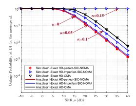
**Fig. 7**: Comparison of the outage probability at  $D_1$  versus transmitting SNR for the cases of perfect and imperfect SIC  $x_2$  with different values of  $\kappa$ .
