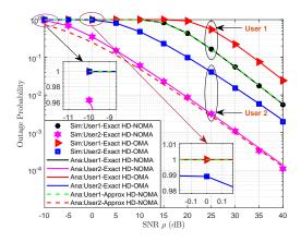
Fig. 4: Outage probability of two users for the PSR protocol versus transmitting SNR.
