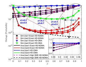
Fig. 5: Outage probability of two users for the PSR protocol versus  $\beta$  and different coefficients of  $a_1, a_2$ .
