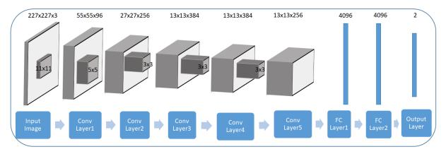
Fig. 2: Modified AlexNet Architecture
