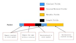
FIGURE 4. Packet assembling process.
