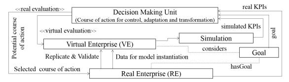
Figure 1: Model Based Digital Twin.
