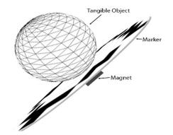
neodymium magnet (20x5mm), providing up to 5kg of pulling force, is attached underneath the centre of the platforms which provides the ability to stick yet freely move the object around on painted steel whiteboards.
