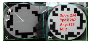
Fig. 5: Determination of captured marker's positional and rotational information
